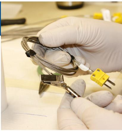
Suitable for measuring air temperatures. Some hand-held probes are designed to measure ambient air temperature, while other models monitor internal temperatures and include a clip for attaching the sensor inside freezers, coolers or ovens. Make sure to check each model for usage, recommendations and maximum temperature limits.
